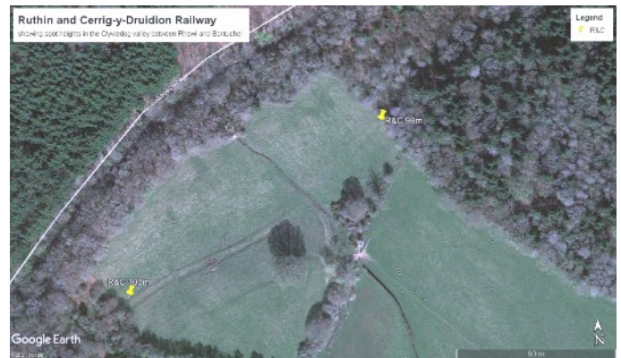
A section of the track bed between Rhewl and Bontuchel. The 'pins' mark the ends of the visible works with spot heights of 98 m (upper right) and 100 m (lower left).
