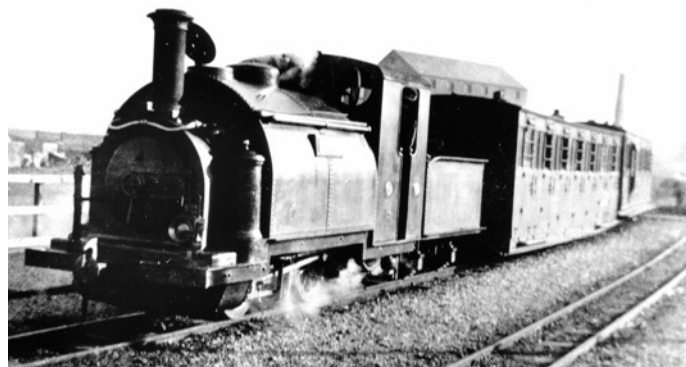
Prince , fitted with chopper couplings, at Portmadoc New with a train comprising an FR Ashbury (21 or 22) and a WHR Pickering, because of braking restrictions, Pickering No. 4 - Summer 1923 - G.H.W. Clifford - WHHG 39 (Arch 0308)
