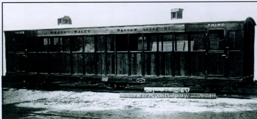
6-wheeler, maker's photo. It was delivered varnished but may have ended up maroon. There is no evidence of this vehicle ever carrying a device.
