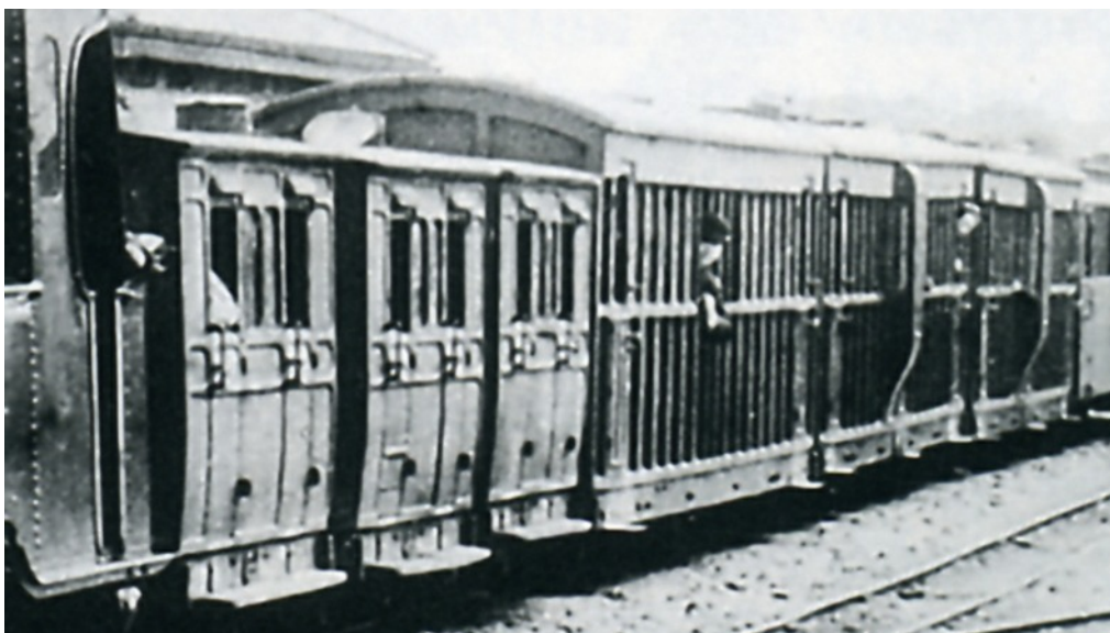
The Railway's three Ashbury 4-wheel carriages are seen here with all three of their Cleminson 6-wheel carriages. Two of the 4-wheelers and one of the 6-wheelers (one of the two brake composites seen here) made up the train involved in 1884 accident north of Snowdon Ranger - Symons Gems of Wales 1892
