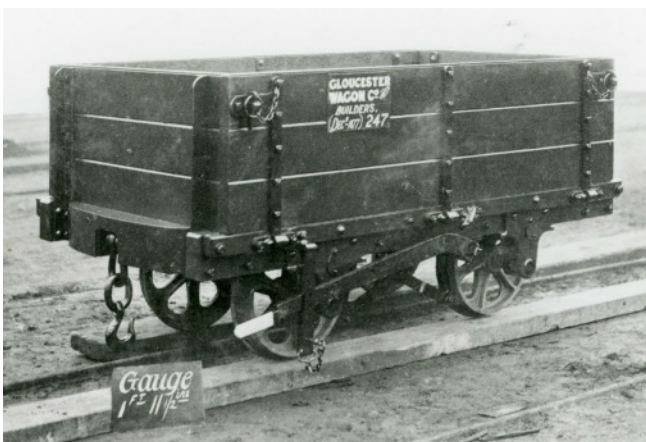
Figure 1 (left) - Maker's photograph of a drop-sided wooden slate wagon for the NWN GR - Gloucestershire Records Office D 4791/16/1
