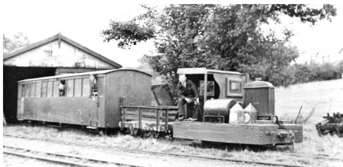
One of Cohen's tractors in process of removing Ashbury 'Corridor' No. 24 (the ex-Buffer Car) from the Dinas carriage shed, completing the outdoors line-up of surviving carriages seen in other photos. J. F. Bolton - 1941 -WHR 78
