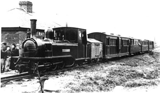
Moel Tryfan with a mixed train at Rhyd-ddu shortly after continuous-brakes were fitted - Arch 4933.
