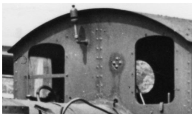
The distinctive group of four bolts mounting the lubricator sight-glass (detail from WHR 8) J.E. Simpson - 1935
